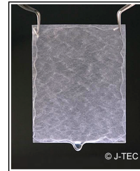
A sample of Fujifilm's micro-needle array (L500 \mu\text{m} x D200 \mu\text{m} )
